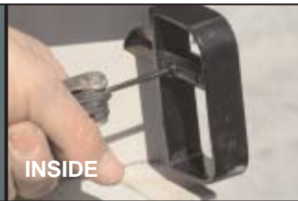
Screw door handle in place
