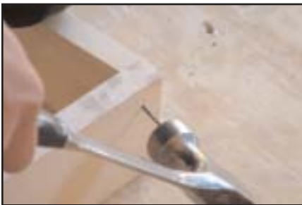
Fasten guides together with 1 1/2" finish nails
